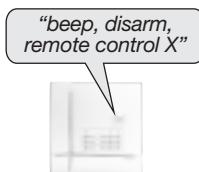
3. The remote control LED lights up a steady green for 1.5 s to confirm.
